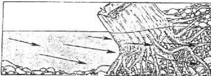
Lateral Scour Pool around Root Wad
